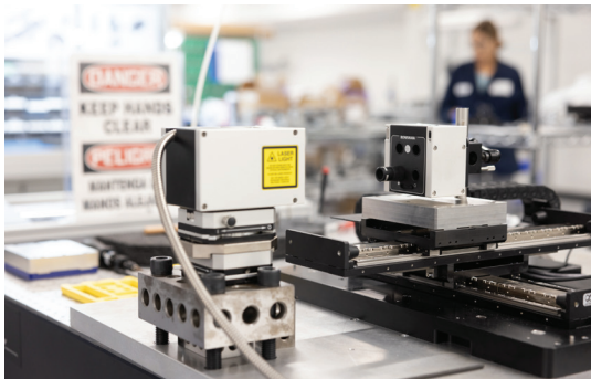
Laser Interferometer test station
